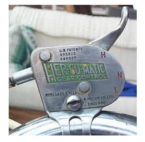
*Postscript:* During the 1950's Hercules hubs were produced which were Sturmey-Archer AW clones. Here is an example of a Her-cu-matic gear control made for three-speed Hercules hubs circa 1958. Note that it displays the same Sturmey-Archer patent numbers.
