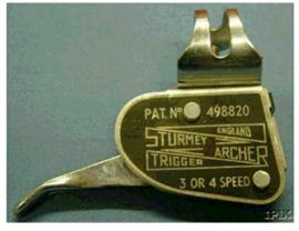
Model GC2. Introduced 1948-9 for 3 or 4 speed hubs with original patent number 498820.
