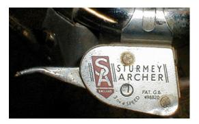
Model GC2. 1950-3. Variant of the above with STURMEY ARCHER in black lettering. Note that the writing on the medallion specifies below the handle bar mounting, but the letter in the gear window (L) is inverted for viewing above the bar.
