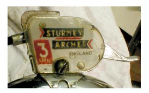
Trigger with plastic cover. The design is similar to the triggers above but the print is located on the plastic cover and not the medallion. Fixing screw through body. Introduced after 1966.
