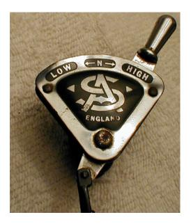
A precursor to the trigger shifter is the quadrant shifter (GC1). This typically was used for the Sturmey-Archer K series hubs. It had three positions Low, N (Normal) and High. It was mounted on the top tube.
