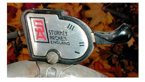
A version with plastic cover but without the large red 3 speed label was in use from approximately 1971 until the mid-1970s.
